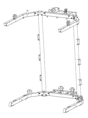
If you tighten every bolt firmly at first, it may result in the distortion of the finished product. To avoid this, tighten bolts lightly until the main frame is assembled and leveled then fasten the all bolts firmly.
