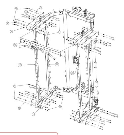
If you tighten every bolt firmly at first, it may result in the distortion of the finished product. To avoid this, tighten bolts lightly until the main frame is assembled and leveled then fasten the all bolts firmly.
